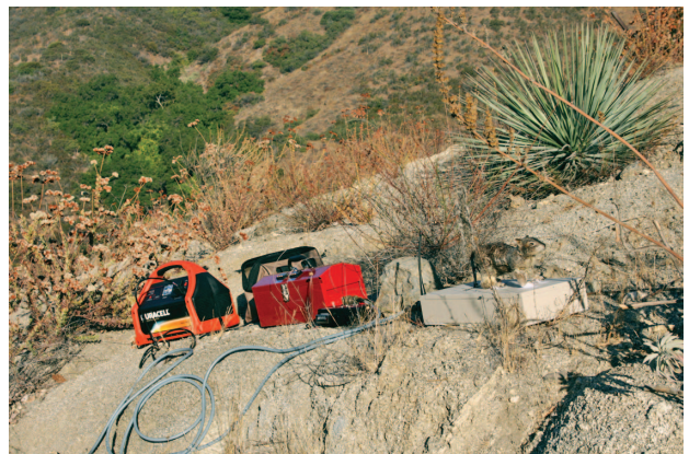
Figure 6. Prototype field-ready robotic squirrel sits on hillside in SMER outside the town of Fallbrook, California. Red toolbox contains thermal controllers and orange box contains power inverter. (Photo courtesy of S. Joshi.)
