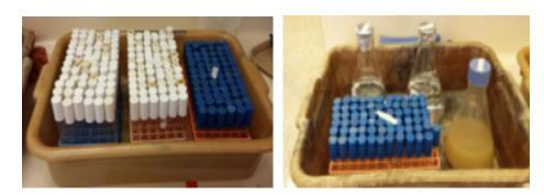
B) 75% filled primary items are spaced in appropriate plastic secondary container.
