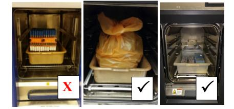
D) Appropriate plastic secondary containers are properly placed inside the autoclave equipment.
