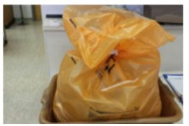
C) Autoclavable bags are filled to only 75% of their holding capacity and placed inside appropriate plastic secondary container. The bag opening should be at least 3 finger widths to allow steam to penetrate inside the bag.
